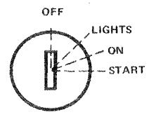
Key operated, 4 position switch. To start engine, turn key fully clockwise to START position and hold. Return key to ON position immediately engine has started. To stop engine, turn key counter-clockwise to OFF position. To illuminate both headlamp and taillight, turn key to LIGHTS position.
