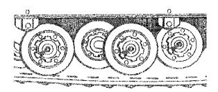
To grease the inner side bogie wheels, tilt vehicle on its side and apply pressure on track to expose grease fittings.
