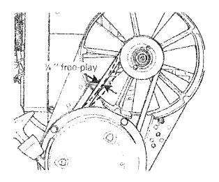
If belt seems damaged or if tension is incorrect, contact your dealer immediately.
