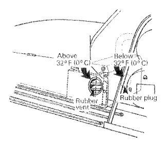
If temperatures below 32° F. (0° C.) the rubber plua must block the entry of fresh air and the rubber vent must allow the warm air being emitted from the engine to be directed over the carburetar.
