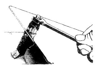
To adjust locking device turn nut in required direction.
