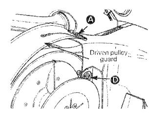
Pull out retaining clip (D) to disengage pin from bracket.
