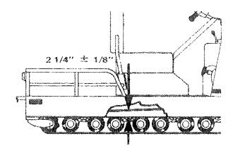
The tension of each track should be 2¼" ± 1 / 8" between top inside edge of track and bottom of footboard.
