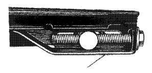
Start engine and allow tracks to rotate slowly. Check if tracks are well centered and turn evenly on the rear sprockets. The distance between track edges and link plates should be equal.
