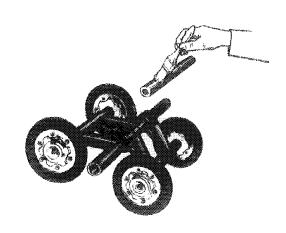
Reassemble entire bogie wheel set, making sure assembly moves freely. Reinstall bogie wheel set. Repeat above steps on remaining bogie wheel sets. Lubricate rear hubs through grease fittings.
