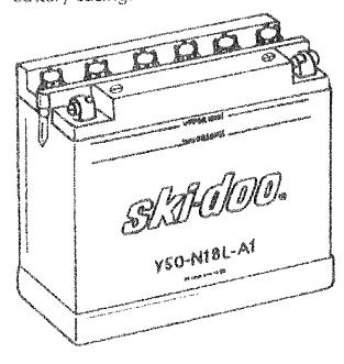
If necessary add distilled water. Battery connections must also be free of corrosion. If cleaning is necessary, remove corrosion using a stiff brush then clean with a solution of baking soda and water. Rinse and dry well.
