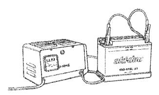
Coat battery terminals with petroleum jelly and store unit in a cool, dry place.
