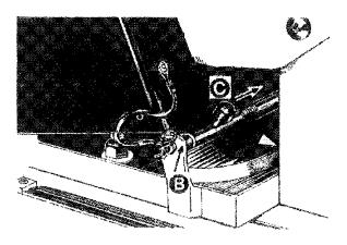
3. Move pulley guard toward front of vehicle to disengage it from front bracket.
